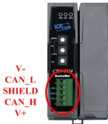
Figure 9-3 CAN-8124 power pin assignments
