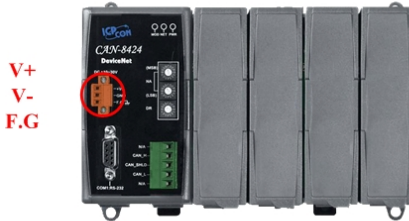
Figure 9-2 CAN-8424 power pin assignments
