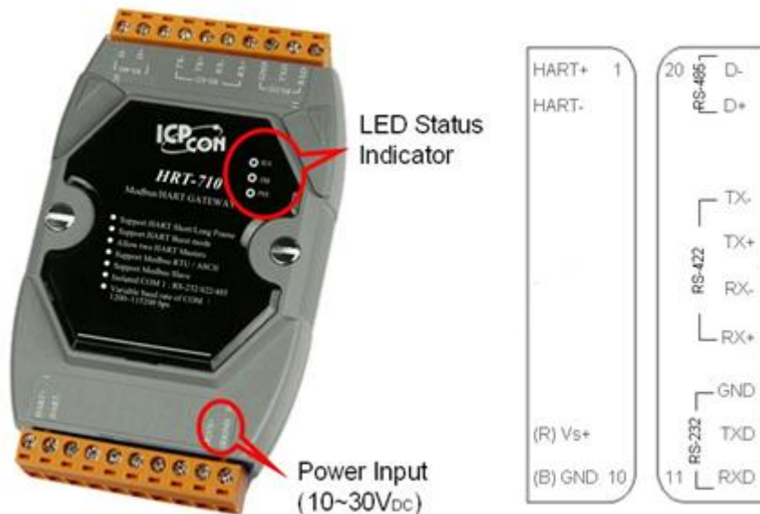
Figure 3.1: Pin assignment of HRT-710
