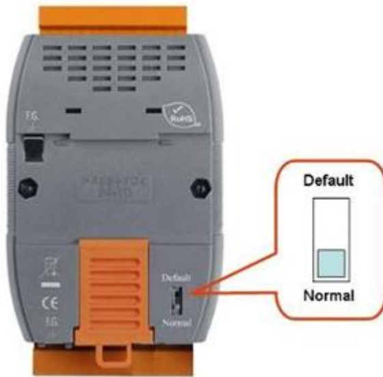
Figure 12-1: DIP Switch of the HRT-710
