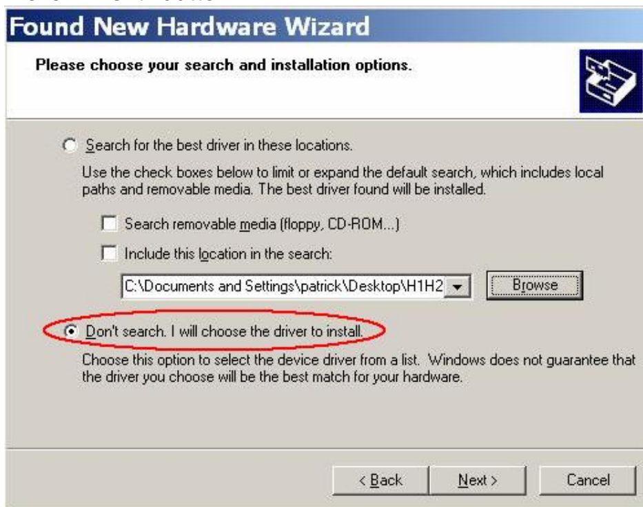
Figure 7.8-1: Driver Installation of I-7565-H1/H2 (1)
