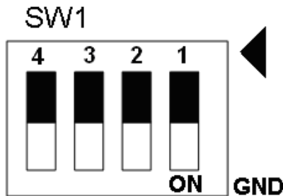
Fig. 3-14 SW1 setting for user controlled signals.
