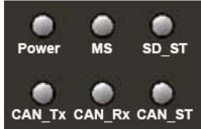
Figure 2-6 LED Assignment of CAN-Logger100
