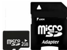
A micro SD card & a micro SD/SD adapter
