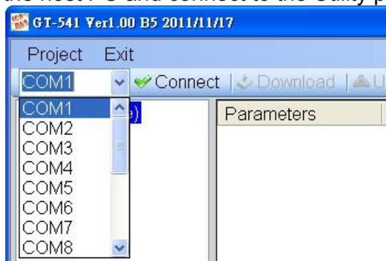
2. Click the “Connect” button to connect to the GT-541. If the connection is failed, check the COM port settings and wiring.
