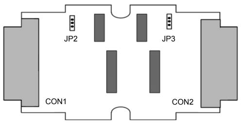
The following connection statuses present the condition if the terminal resistor is enabled (default) or disabled.
