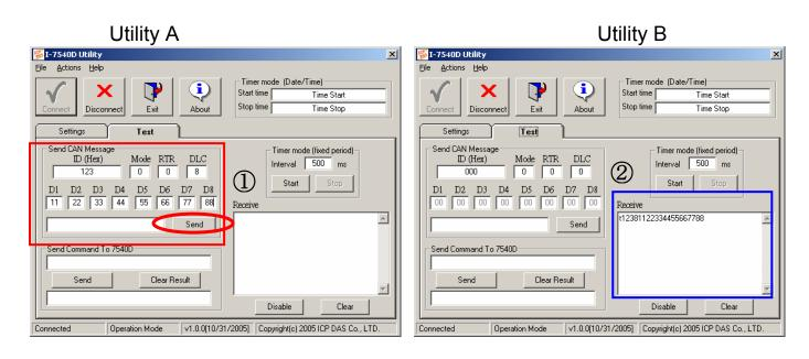
Step5: In "Send command to 7540D" frame, Users can directly type the ASCII command string, "99S","99C","99RA", to get/set the status of the 7540D. The sample picture below is using command, "99S", to get the module status of 7540D.
