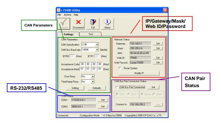
Step5: After connecting with the I-7540D\_A, you can modify the CAN parameters and network status of it. The CAN parameters and network status of I-7540D\_A and I-7540DB are setting as following table.
