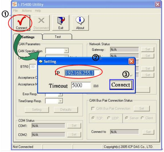
Step4: Click the "Connect" button. If this process is successful, the I-7540D Utility shows the I-7540D\_A communication information as below.
