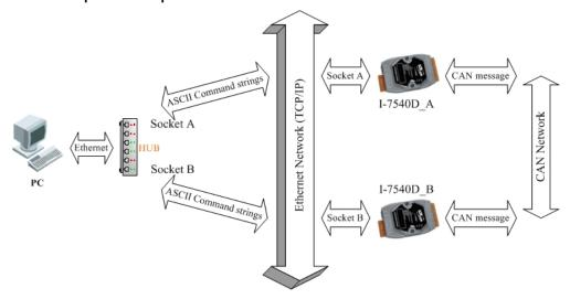
When the I-7540D receives a valid message, with the ASCII strings format from Ethernet port, it converts this message into a CAN message and transmits it into the CAN network. Based on the same reasoning, when a CAN message is received via the I-7540D, the CAN message will be transferred to a message by using the ASCII strings format through the Ethernet port.
